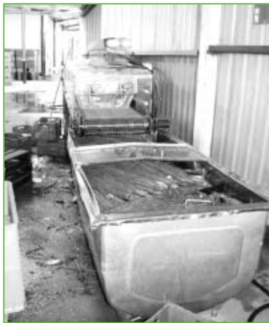
A vegetable washing system using pressure washing and a sanitised water rinse
